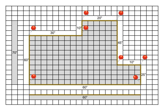
All inside corners are cut with a nominal 1" radius. All outside corners are cut with a 2" radius.
